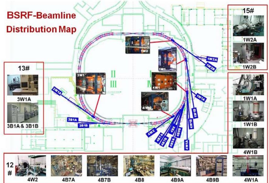
There are 3 experimental halls (12#, 13#, 15#), 5 insertion devices and 14 beamlines and stations in BSRF.
