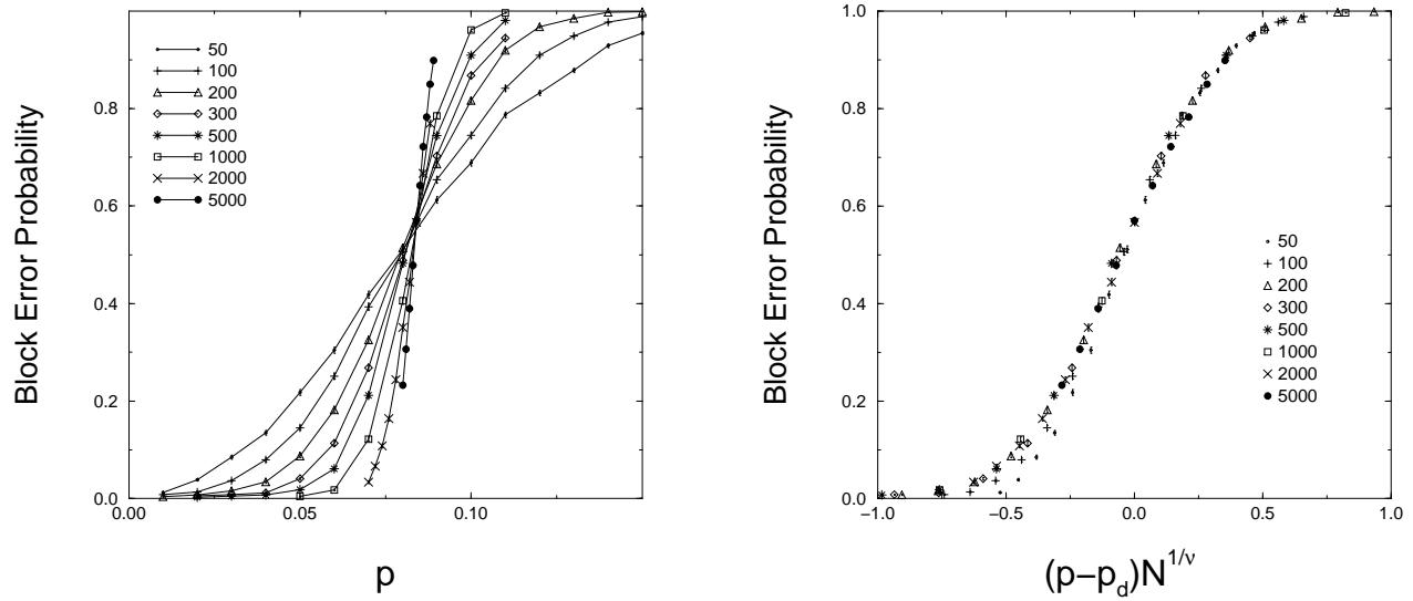
The block error probability for a (6, 3) regular Gallager code for several block lengths (see the legend). On the right the *scaling plot* (see text) for the same quantity.
